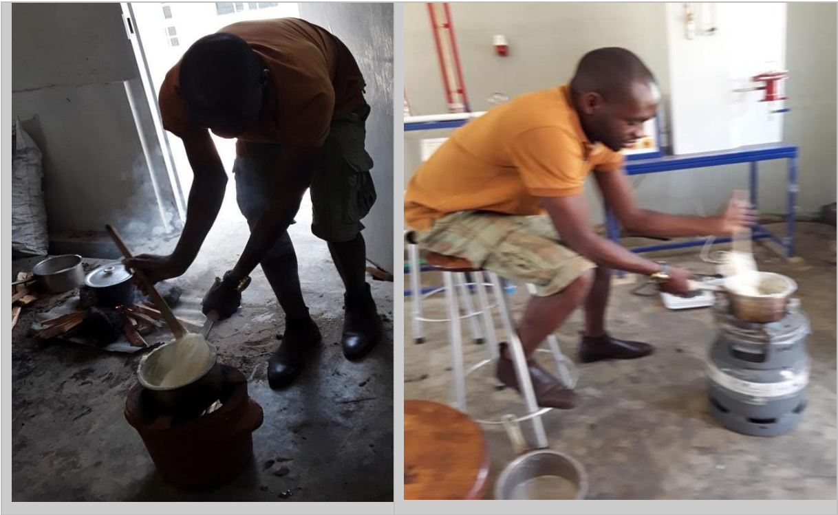
D3: Controlled cooking test for chitetezo mbaula and 3-stone fire
