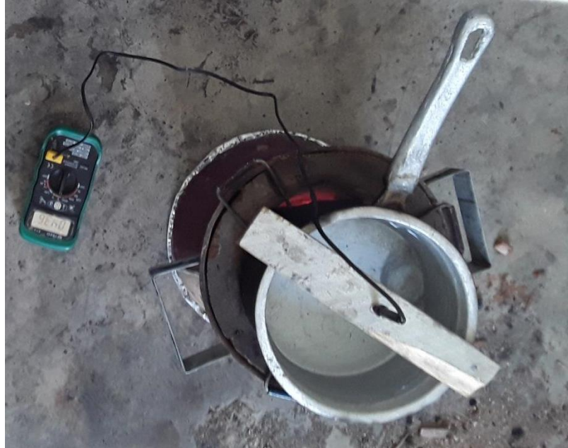
D1: Test rig during WBT for ceramic jiko burning local charcoal. Digital thermal and k-type thermocouple probed into the water are shown.
